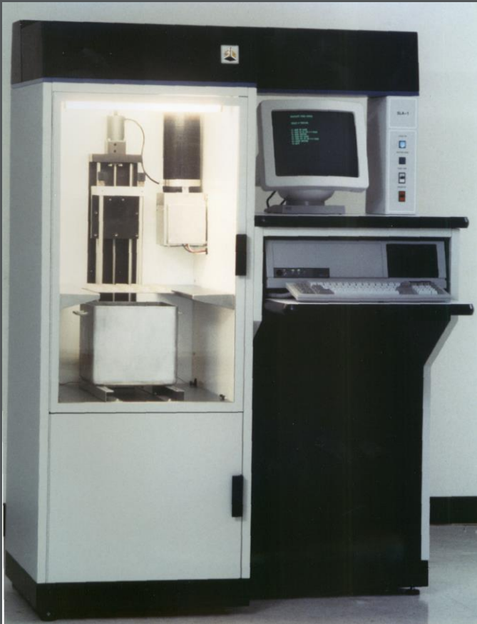
SLA-1, the first commercial prototyping device from 3D Systems
