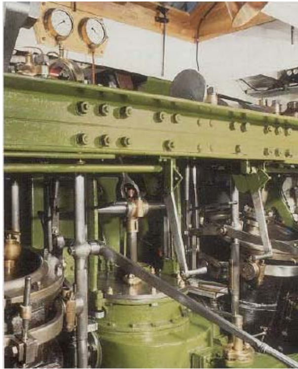
View of engine frame, with portions of the two cylinders and air pump visible below. The long handle is for valve adjustment. Photo: Sächsische Dampfschiffahrt
