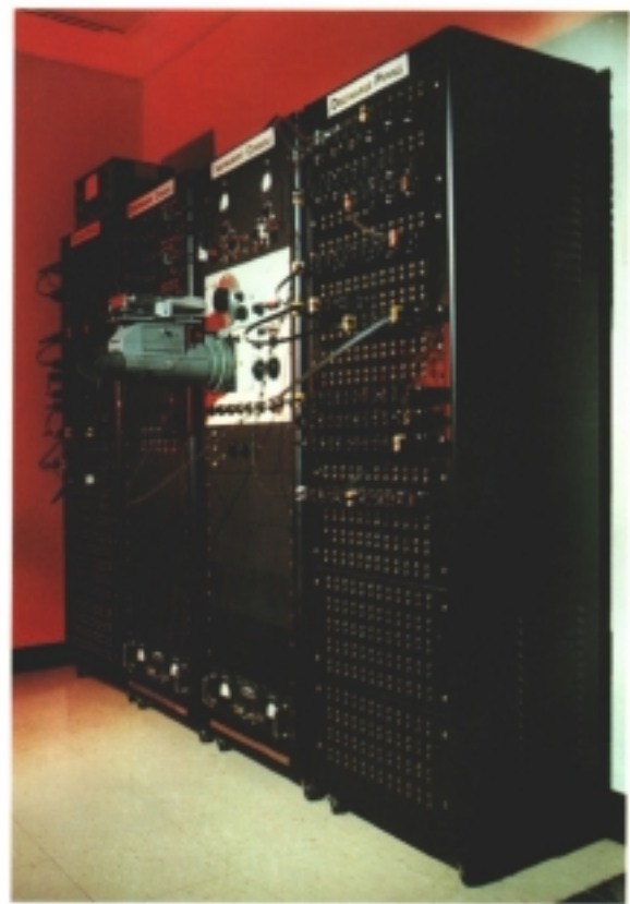
Original analog components, including crankshaft power supply, oscillator, instrument console, and piping coils and capacitors, are mounted for permanent display at SwRI.
