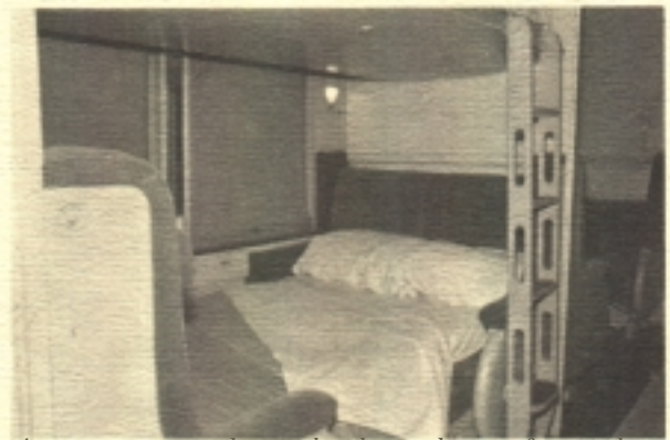
A compartment lower berth made up for night occupancy. Note the ladder for upper berth access. (Photo by J. W. Schroeter)
