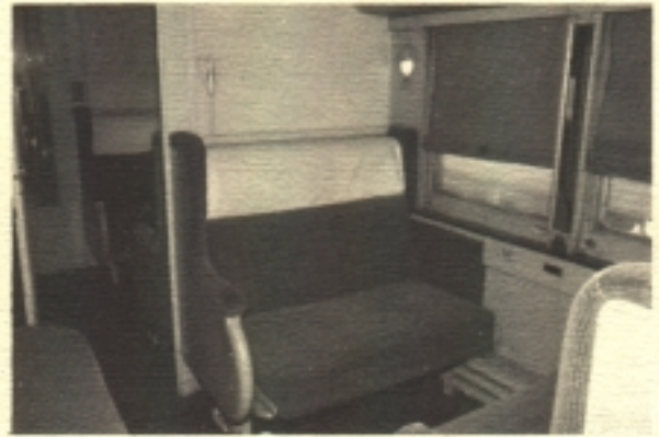
One of Glengyle 's compartments by day. Note the Vapor heat pipes along the baseboard and the individual heat control above the seat. (Photo by J. W. Schroeter)
