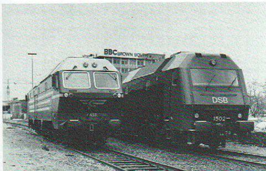
Fig. 27: Diesel-electric locomotive with three-phase drive class ME for Danish State Railways and class Di 4 for Norwegian State Railways.
