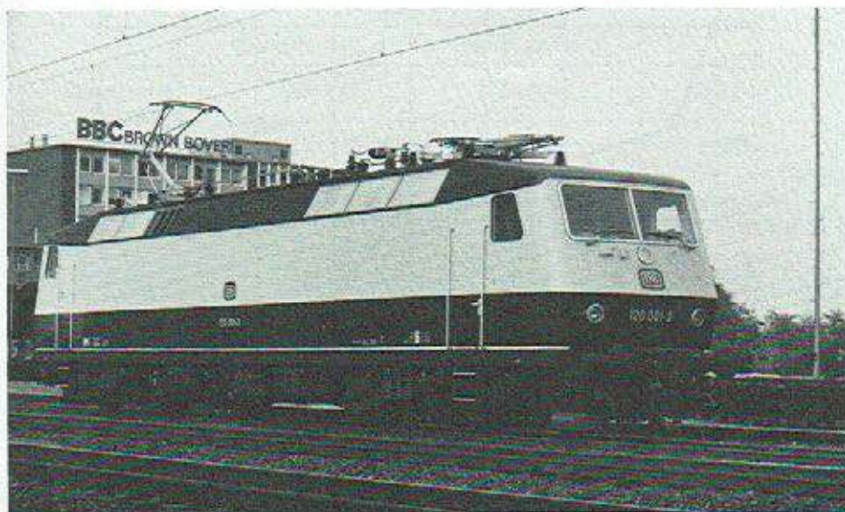
Fig. 16: Electric multi-purpose high-power locomotive class E 120.
