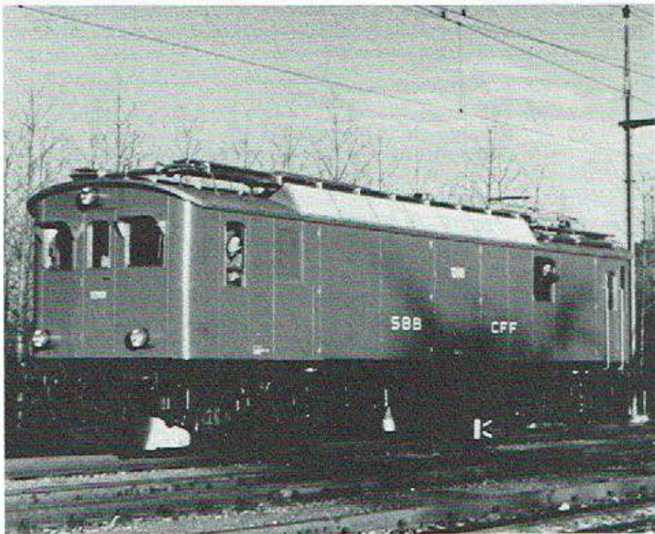
Fig. 8: Experimental inverter locomotive class Be 4/4 of Swiss Federal Railways.
