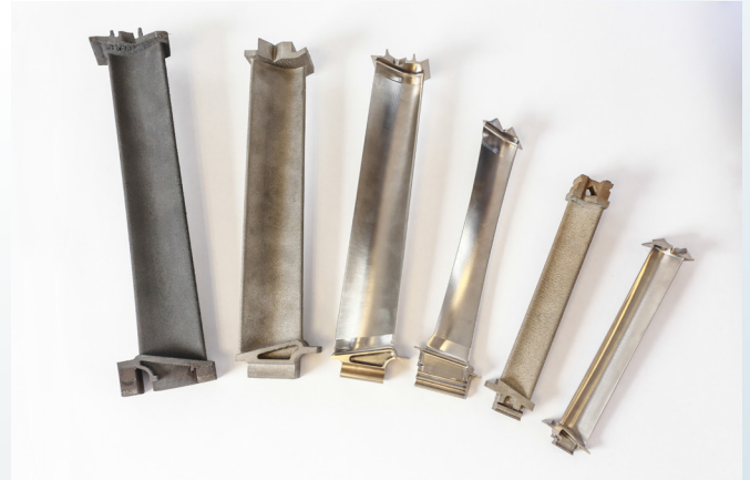
Figure 4. Low pressure turbine blade parts
