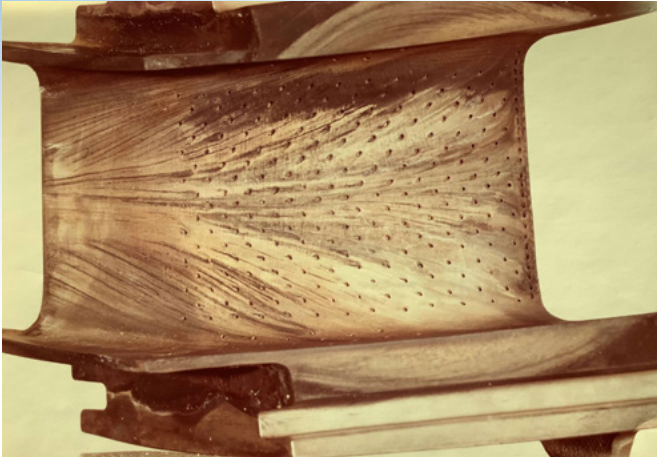
Figure 2. Film-cooled turbine inlet guide vane. (Flow is right to left on the suction surface.)
